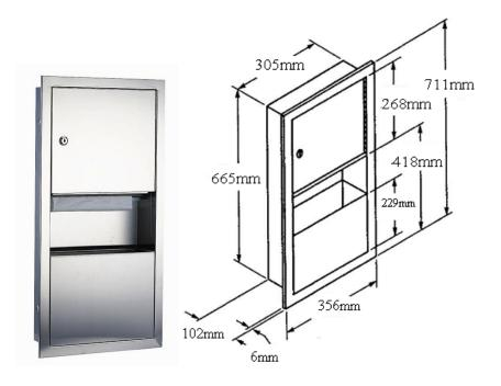
S-137 Fully recessed S-137-15 Semi recessed S-137-20 Surface mounted
