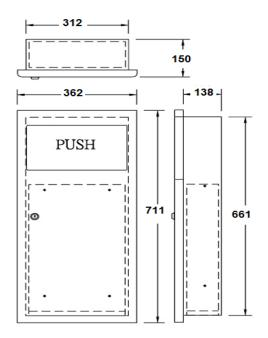
**S-160** Fully recessed **S-160-15** Semi recessed **S-160-20** Surface mounted
