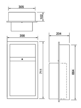
S-165 Fully recessed S-165-15 Semi recessed S-165-20 Surface mounted
