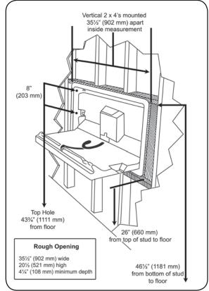
4. Place the unit into the recessed area and insert the screws and flat washers to hold the unit in place. It may be necessary to adjust the level of unit by using a shim on the top right or left side of the unit before tightening securely to the studs.
