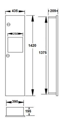
S-1331 Fully recessed S-1331-15 Semi recessed S-1331-20 Surface mounted
