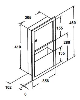
S-135 Fully recessed S-135-15 Semi recessed S-135-20 Surface mounted
